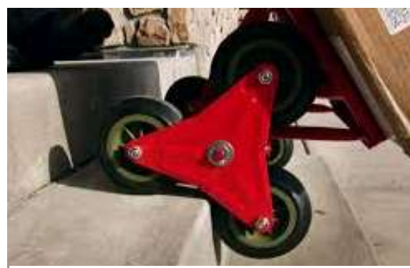
Three wheel stair trolley ‘fridge trolley’ causes less back strain moving heavy items up and down stairs
