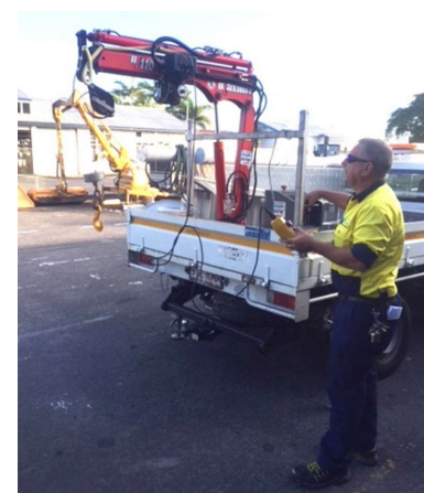
Hiab vehicle mounted crane enables heavy items to be lifted without musculoskeletal strain to the back and shoulders
